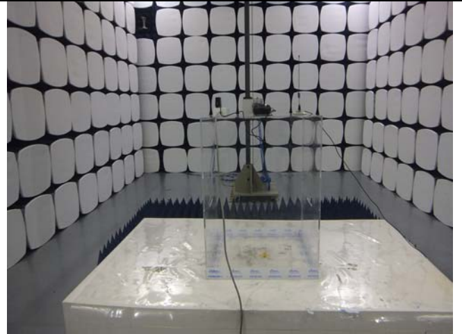
Radiated Spurious Emissions Test Setup Above 1GHz
