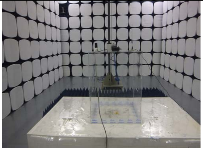
Radiated Spurious Emissions Test Setup Above 1GHz
