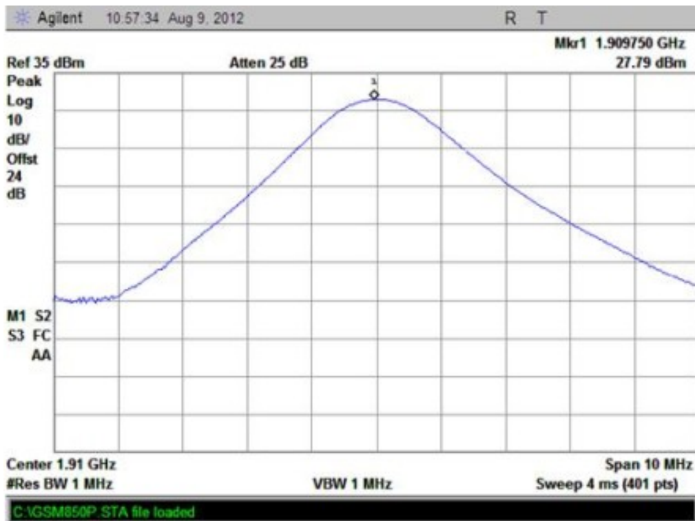
(Plot D3: GPRS 1900MHz Channel = 810)
