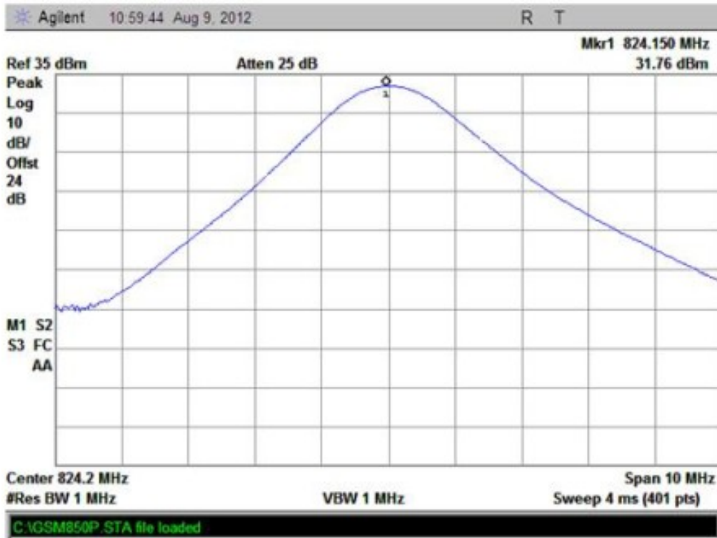
(Plot C1: GPRS 850MHz Channel = 128)
