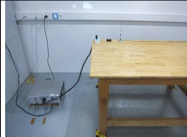
Conducted Emissions Test Setup – Front View
