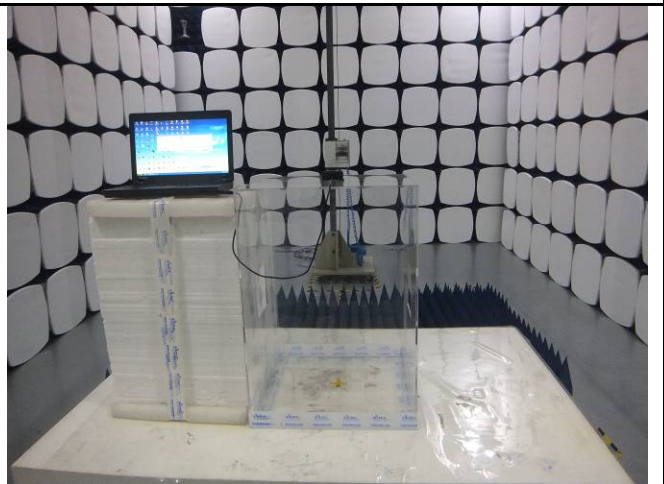
Radiated Emissions Test Setup Above 1GHz
