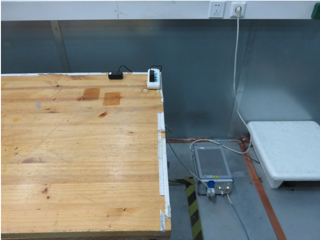
Picture 3 Conducted Emission Test Setup
