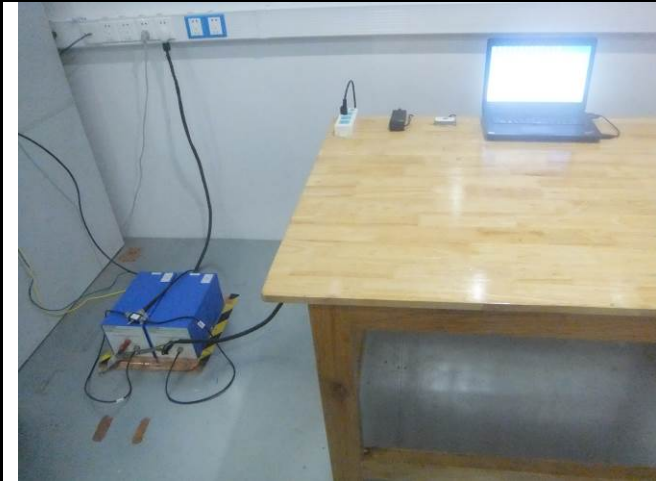
Conducted Emissions Test Setup Front View
