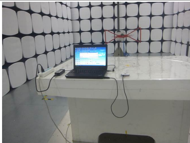
Conducted Emissions Test Setup Front View
