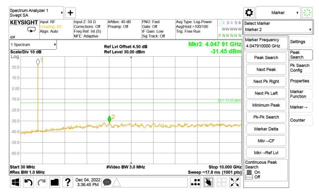
30MHz to 10GHz, Low Channel, Subcarrier (3.75kHz), BPSK, 1@0
