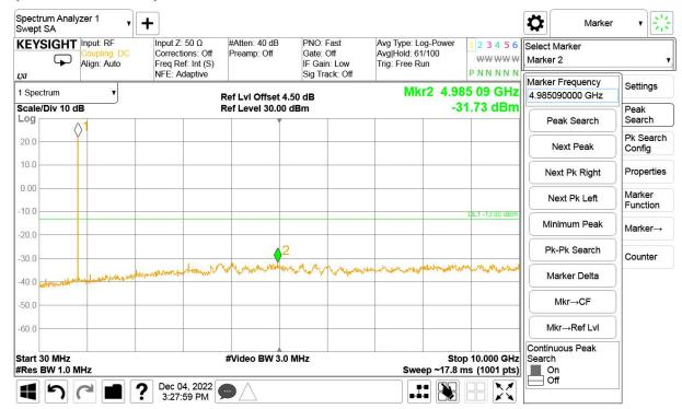
30MHz to 10GHz, Low Channel, Subcarrier (3.75kHz), QPSK, 1@0
