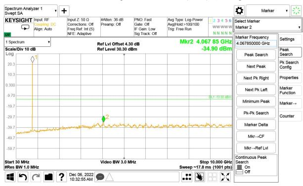
30MHz to 10GHz, High Channel, Subcarrier (15kHz), QPSK, 12@0
