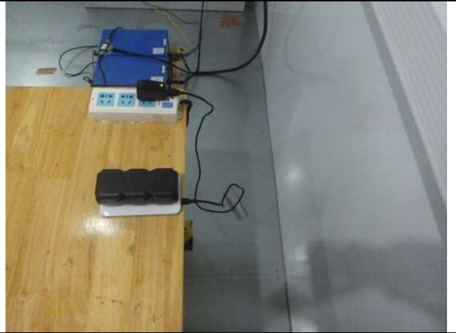
Conducted Emissions Test Setup – Side View
