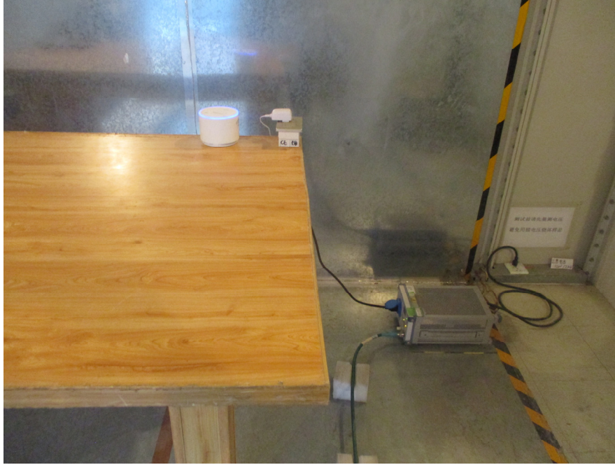
Conducted Emissions - Rear Side
