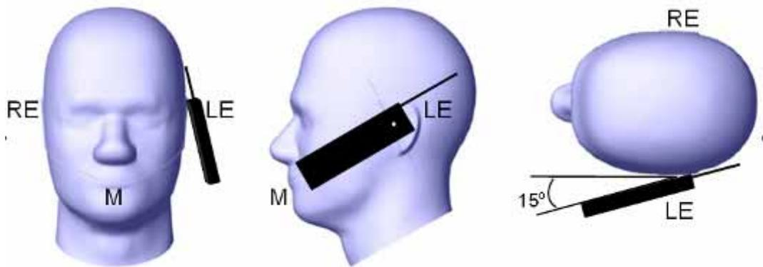
**Test positions for body-worn and other configurations**
