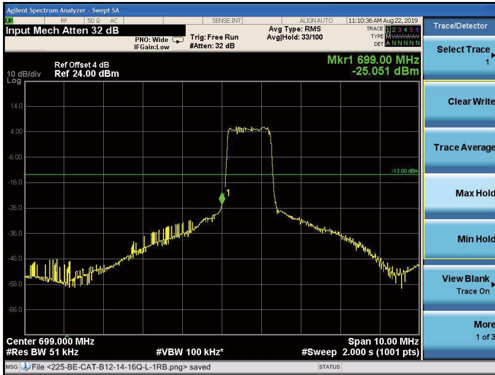
Low Channel-1.4MHz Bandwidth-6RB-16QAM
