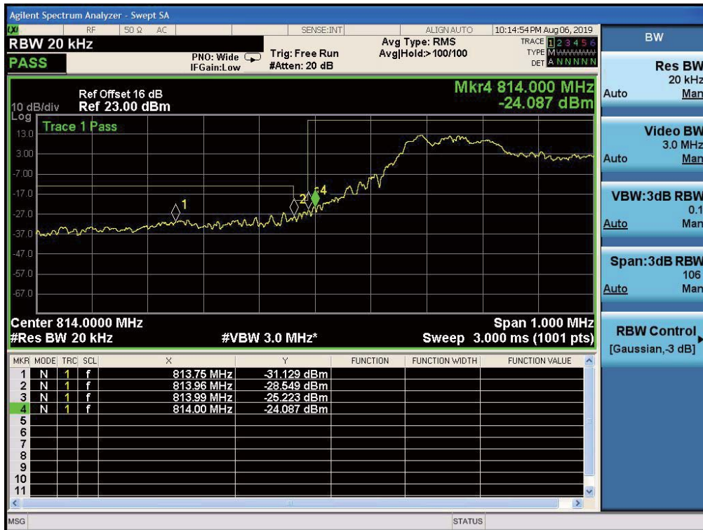
Band26-Low Channel-1.4MHz Bandwidth-1RB-QPSK
