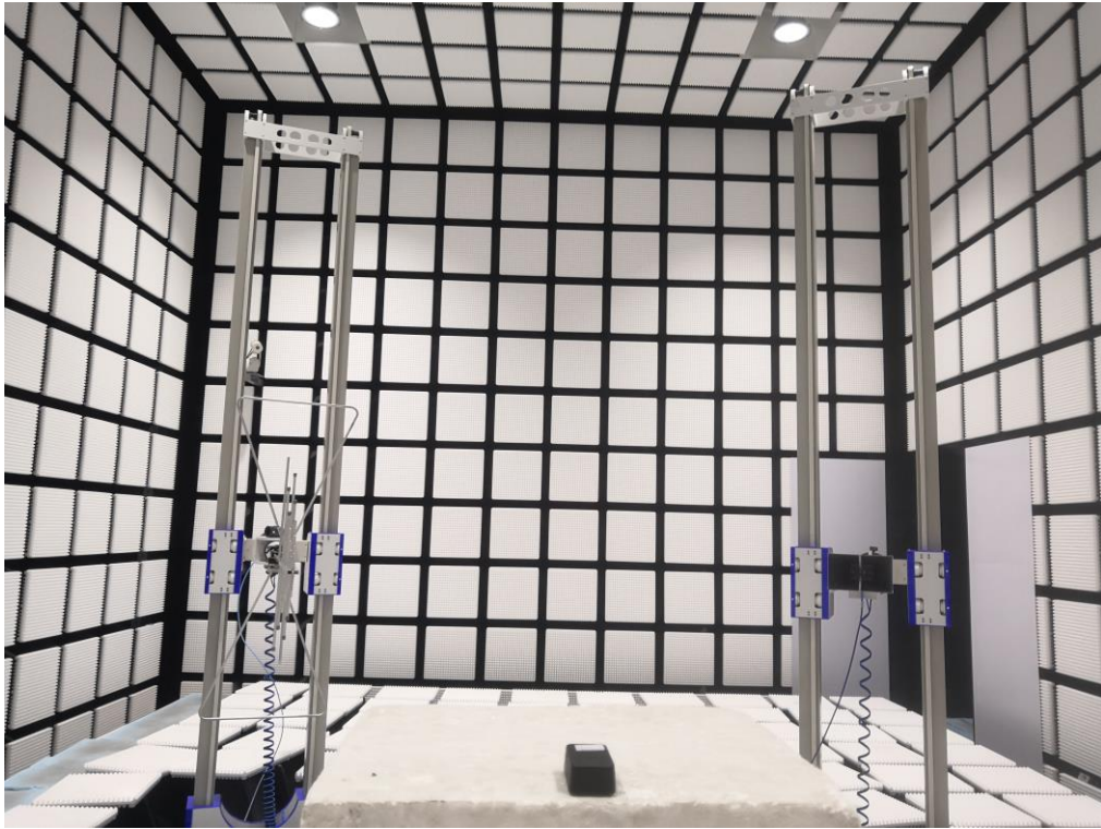
Pic1. Radiated spurious emission (Above 1GHz)
