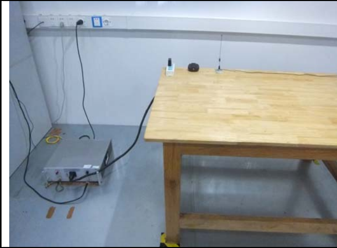
Conducted Emissions Test Setup – Front View
