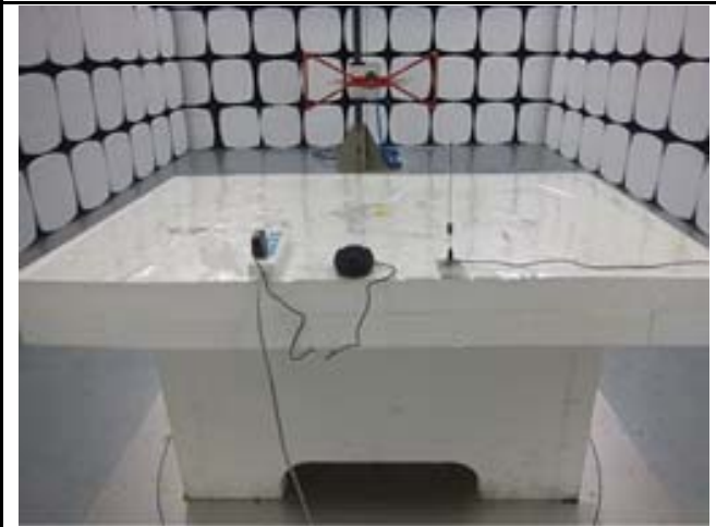
Radiated Emissions Test Setup Below 1GHz
