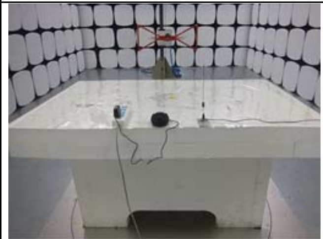
Radiated Emissions Test Setup Below 1GHz
