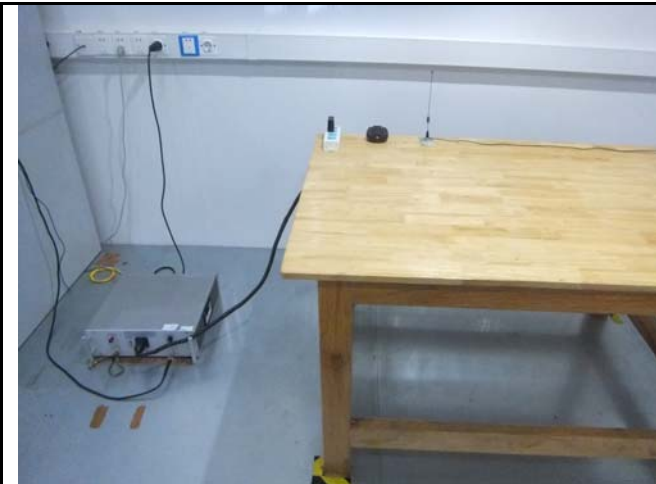
Conducted Emissions Test Setup – Front View
