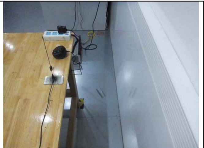
Conducted Emissions Test Setup – Side View
