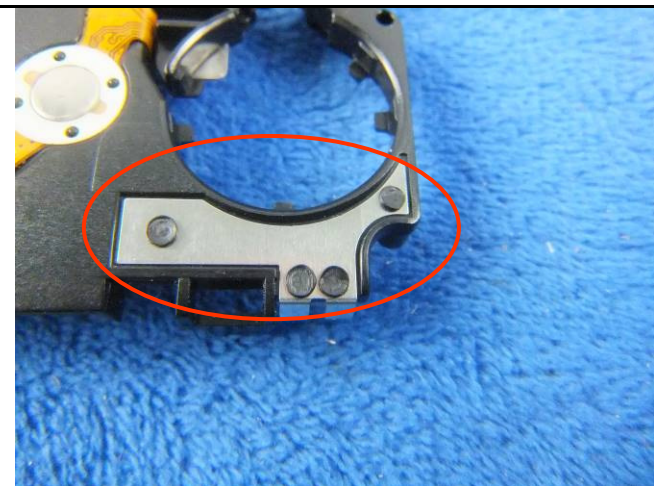
WIFI - Antenna View
