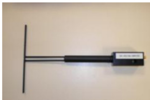
Figure 1 – Satimo COMOSAR Validation Dipole
