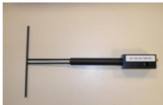
Figure 1 – Satimo COMOSAR Validation Dipole
