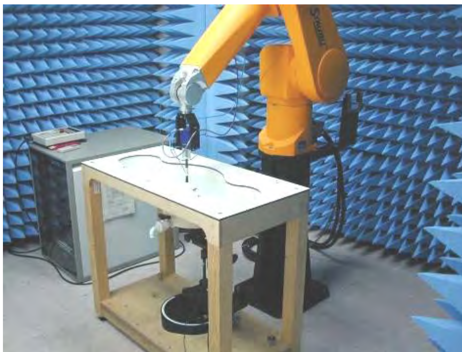
Fig.1 Photograph of the SAR measurement System
