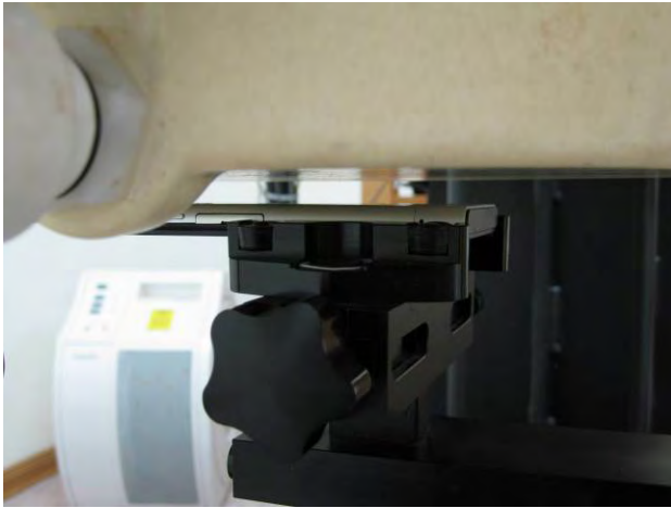
Fig.3 Body worn- EUT rear to flat phantom and distance between flat phantom and mobile phone is 1 cm.
