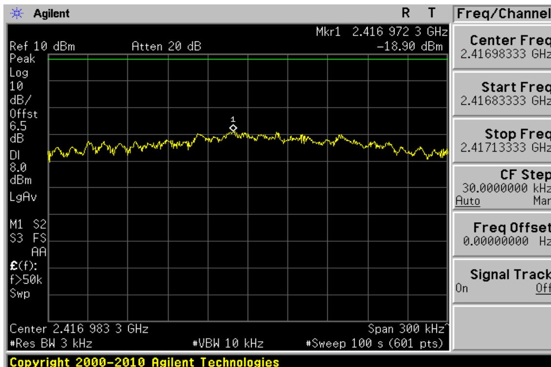
**Power Spectral Density Test Plot (CH-Mid)**
