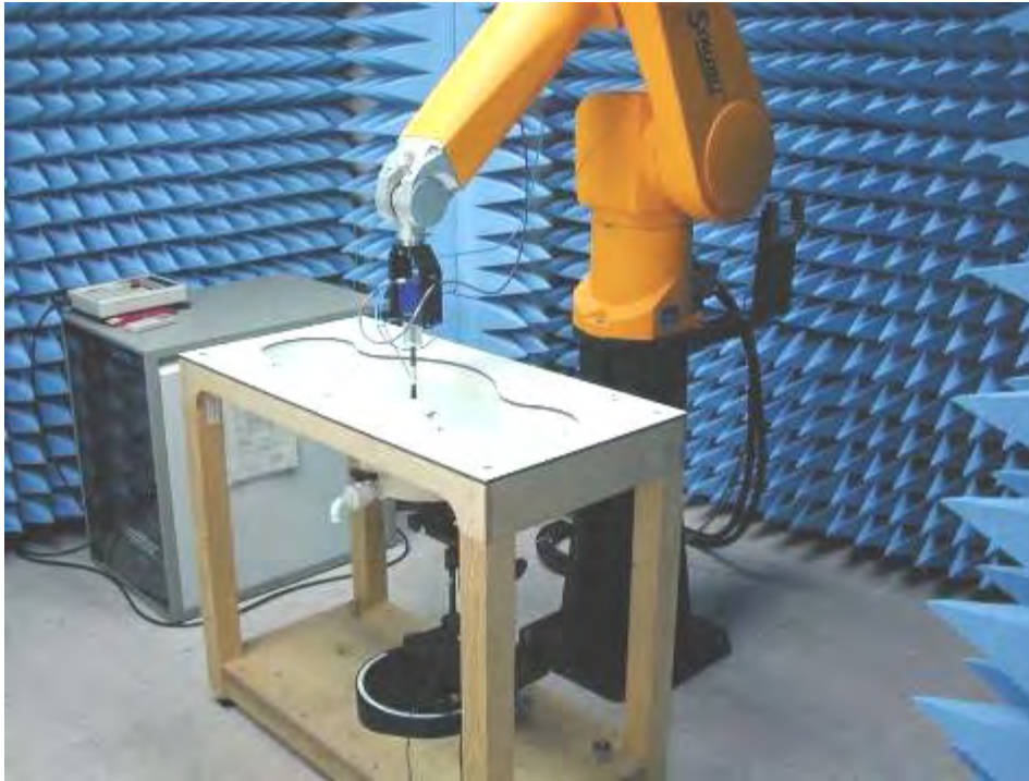
Fig.1 Photograph of the SAR measurement System
