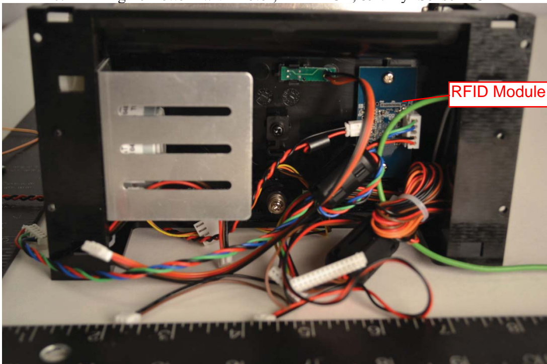
6. Engine Bottom with motor, RFID PCB, & Vinyl Sensor PCB
