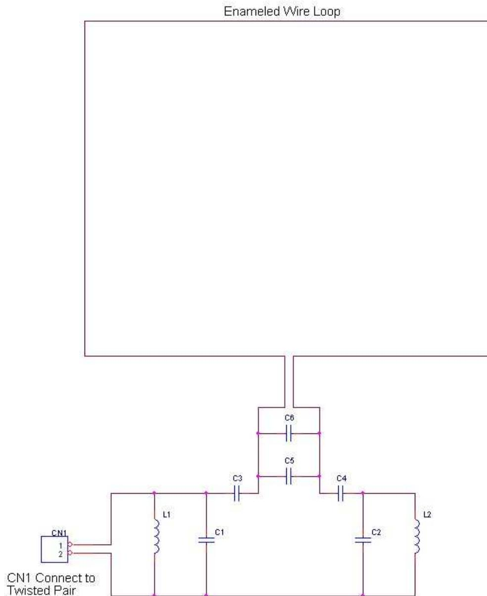
This antenna is a single-loop transmit/receive antenna with pre-set matching electronics for a transmitter frequency of 13.56MHz and impedance of 50Ω.
