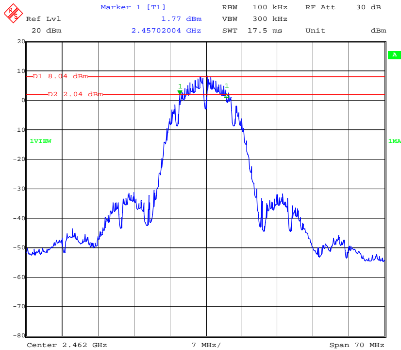
6dB Bandwidth Plot (Channel 11) – 802.11b mode
