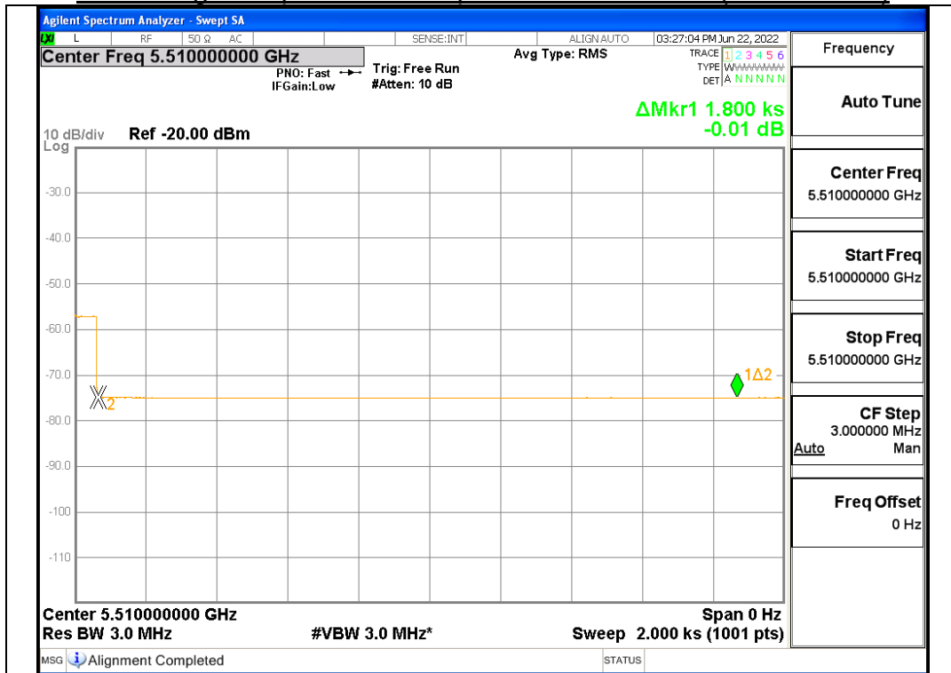
Monitoring live spectrum – Elapse time 30 minutes (40 MHz BW)
