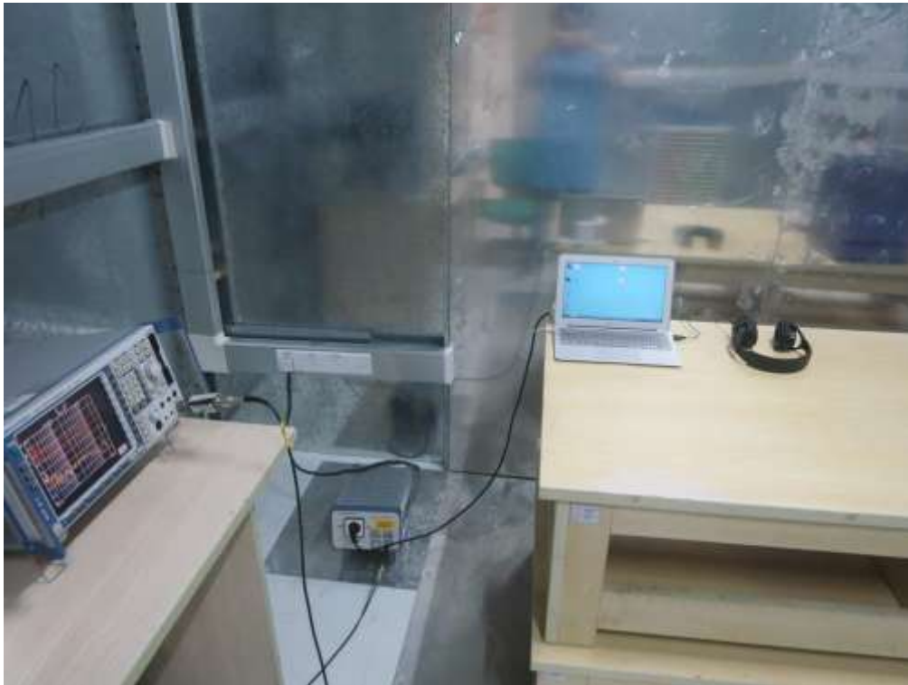
FCC RADIATED EMISSION TEST SETUP
