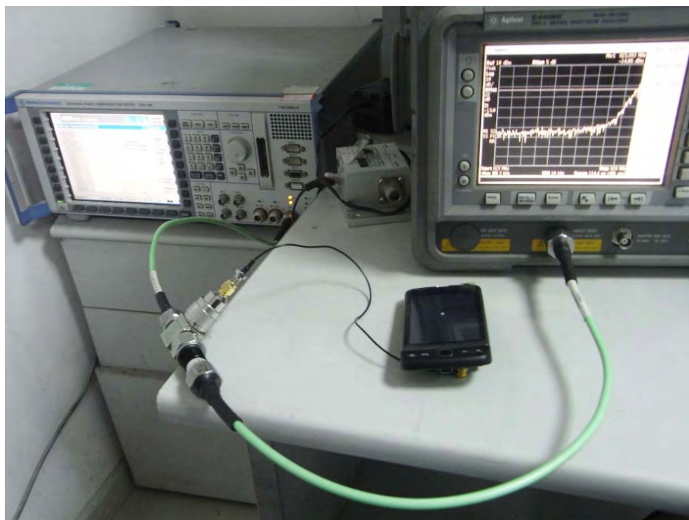
CONDUCTED SPURIOUS EMISSION TEST SETUP
