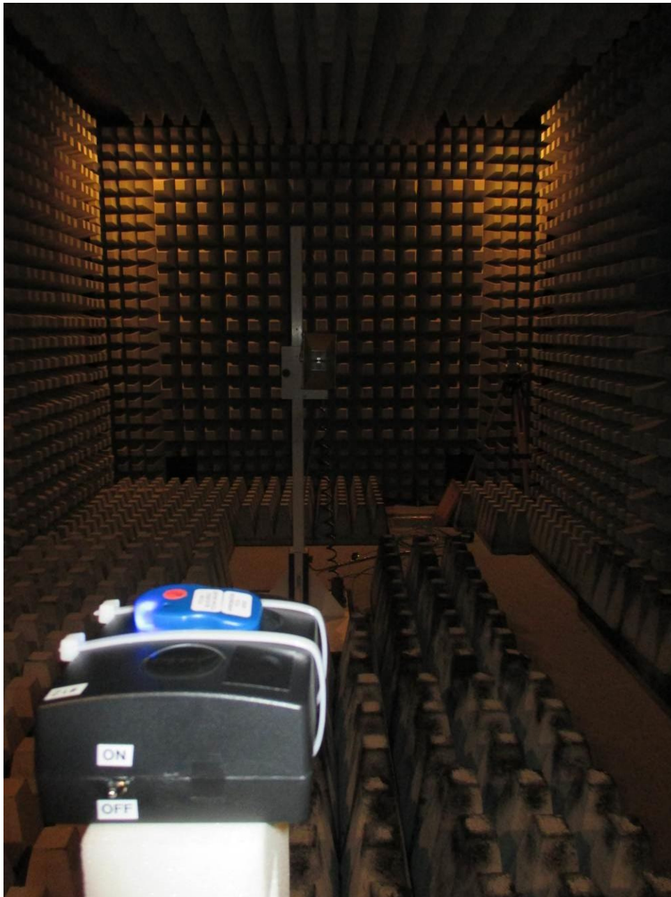
154064_06.jpg: Test setup Blue Frog- Radiated emission > 1 GHz (fully anechoic chamber)
