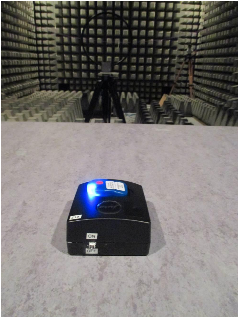
154064_02.jpg: Test setup Blue Frog- Radiated emission < 1 GHz (fully anechoic chamber)
