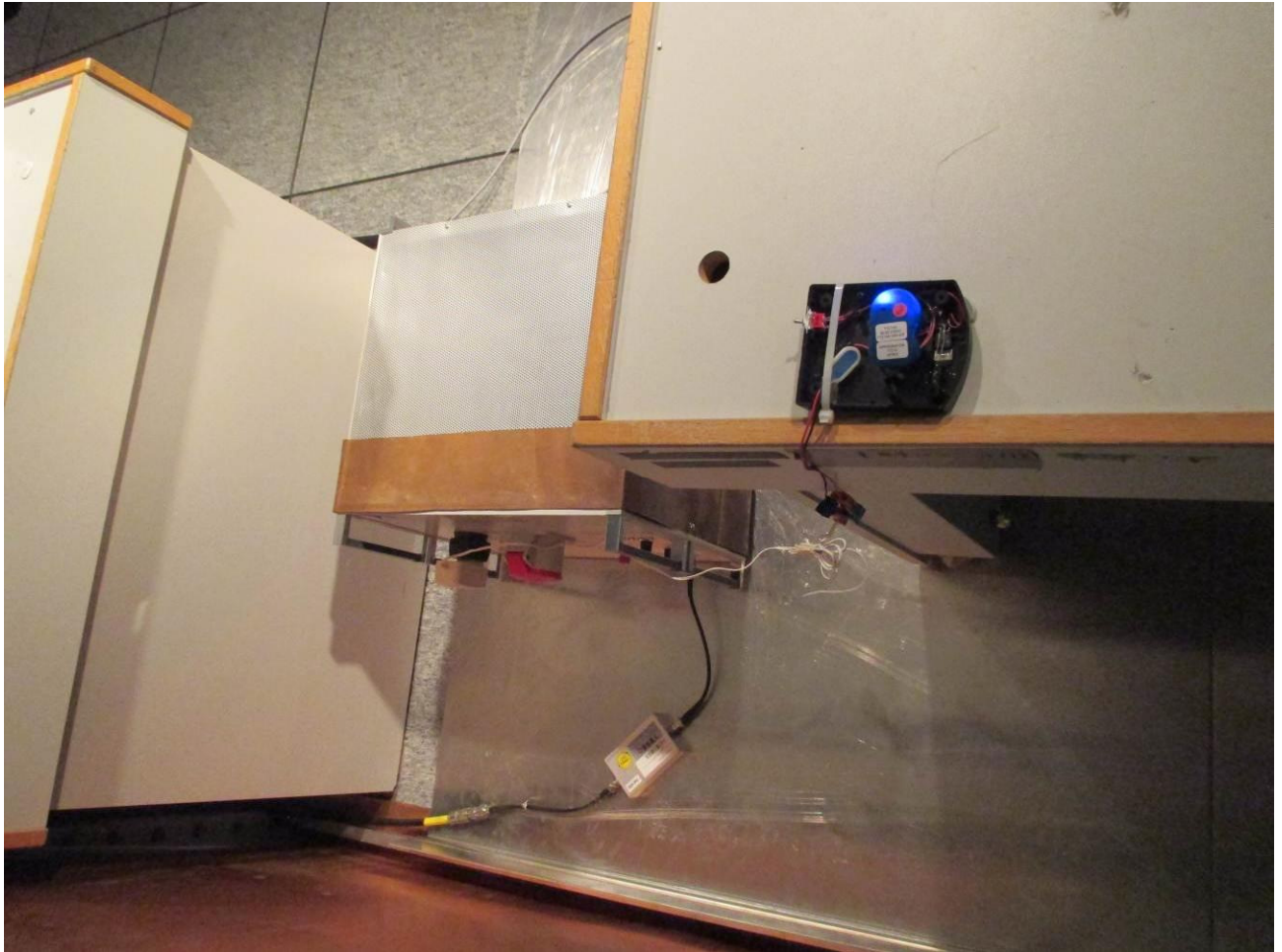
154064_10.jpg: Test setup – conducted emissions on power supply lines (Blue Frog)
