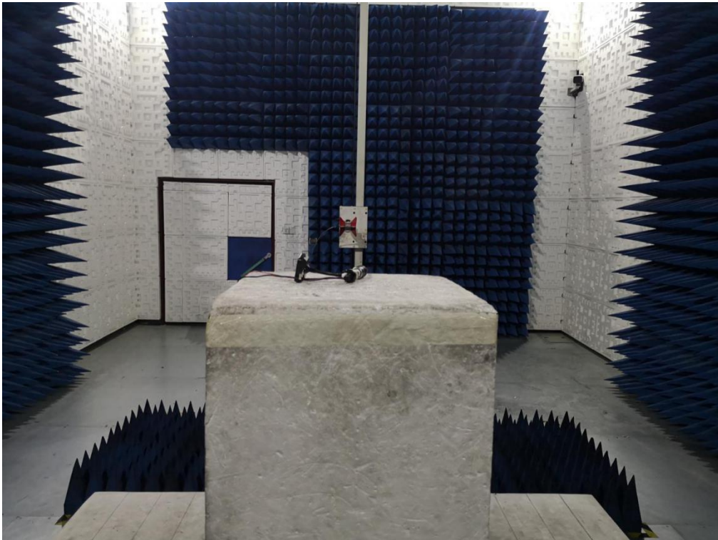
RADIATED EMISSION TEST SETUP ABOVE 1GHZ
