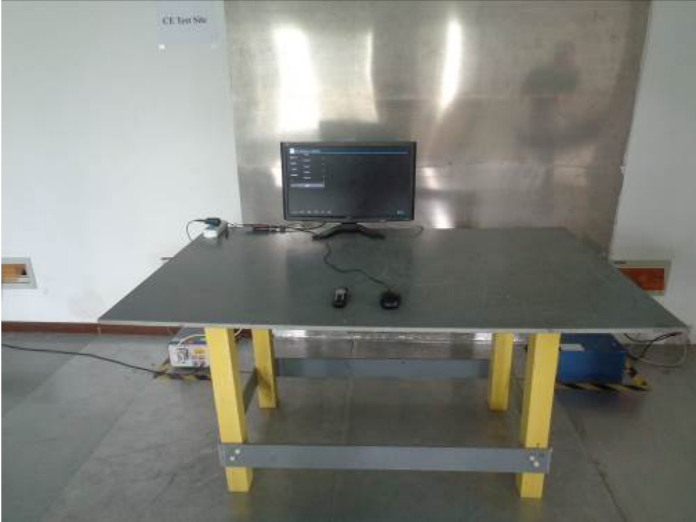
Conducted Emissions Test Setup – Front View
