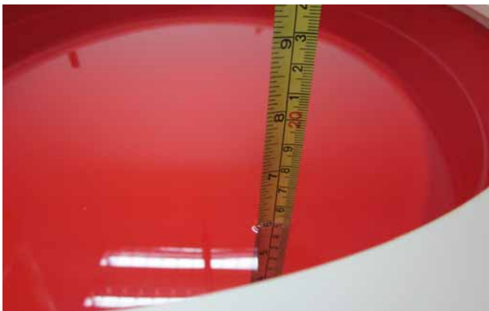
Figure 4.4: Liquid depth in the Flat Phantom
