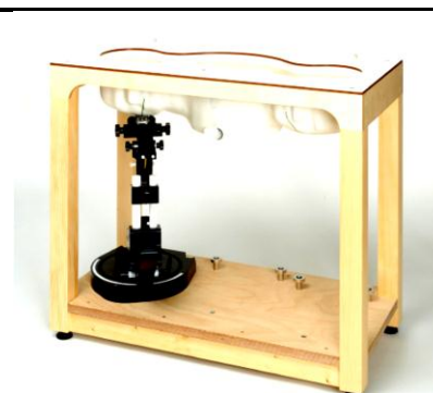
Fig 5.3 Photo of SAM Phantom
