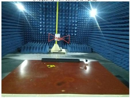
**RADIATED EMISSION TEST** (Frequency above 1GHz)
