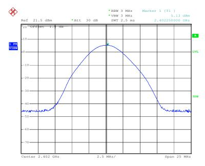
Test mode: GFSK Test channel: Middle
