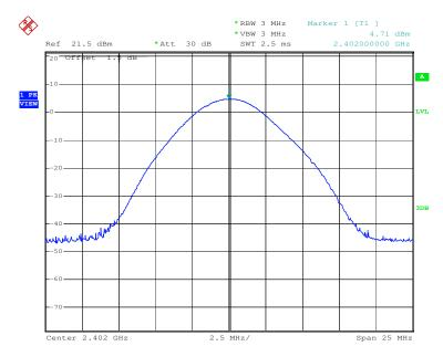
Test mode: 8DPSK Test channel: Middle
