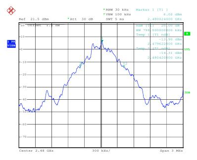
Test mode: π/4DQPSK Test channel: Lowest
