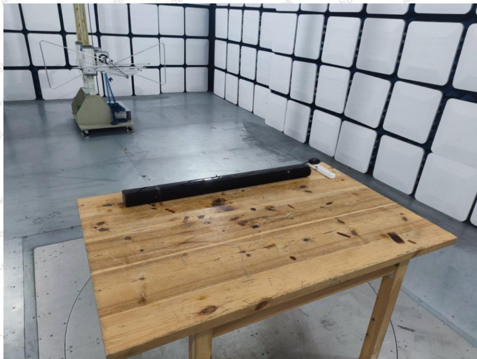
Photo of Radiation Emission Test
