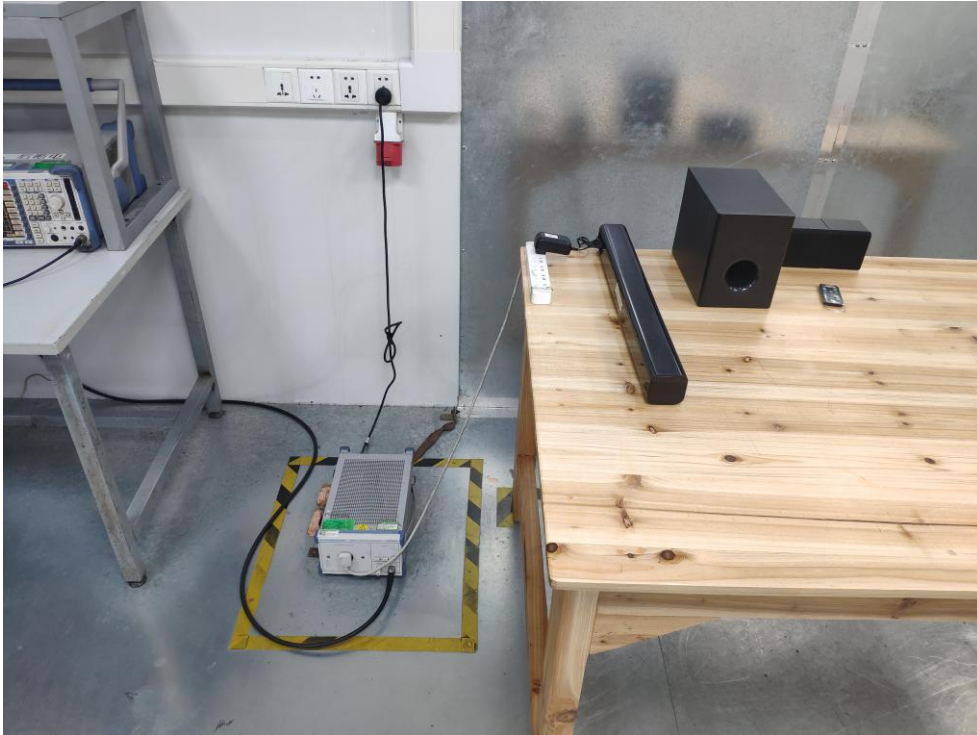
Photo of Power Line Conducted Emission Test
