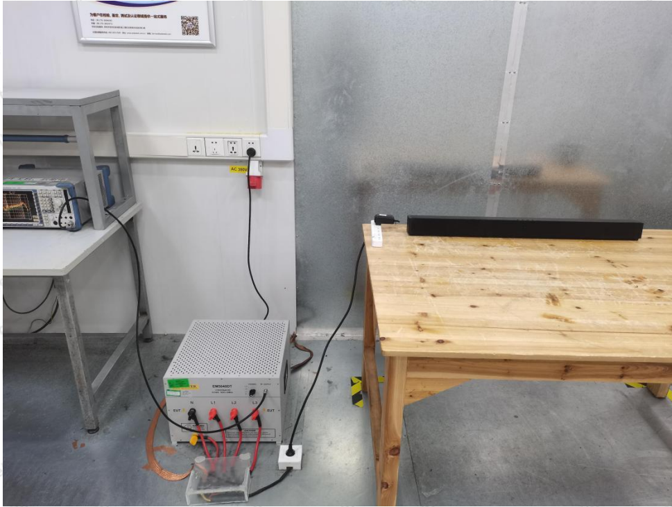
Photo of Conducted Emission Measurement
