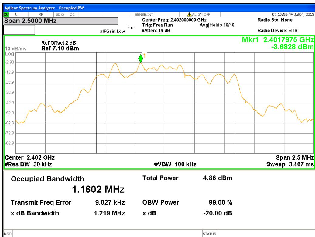
20 dB Bandwidth @  $\pi/4$ DPSK mode channel 39
