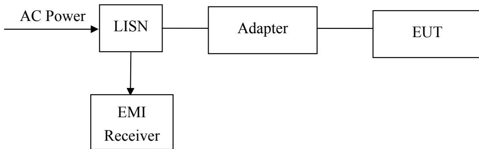
**The test procedure was according to ANSI C63.4/2003.**
