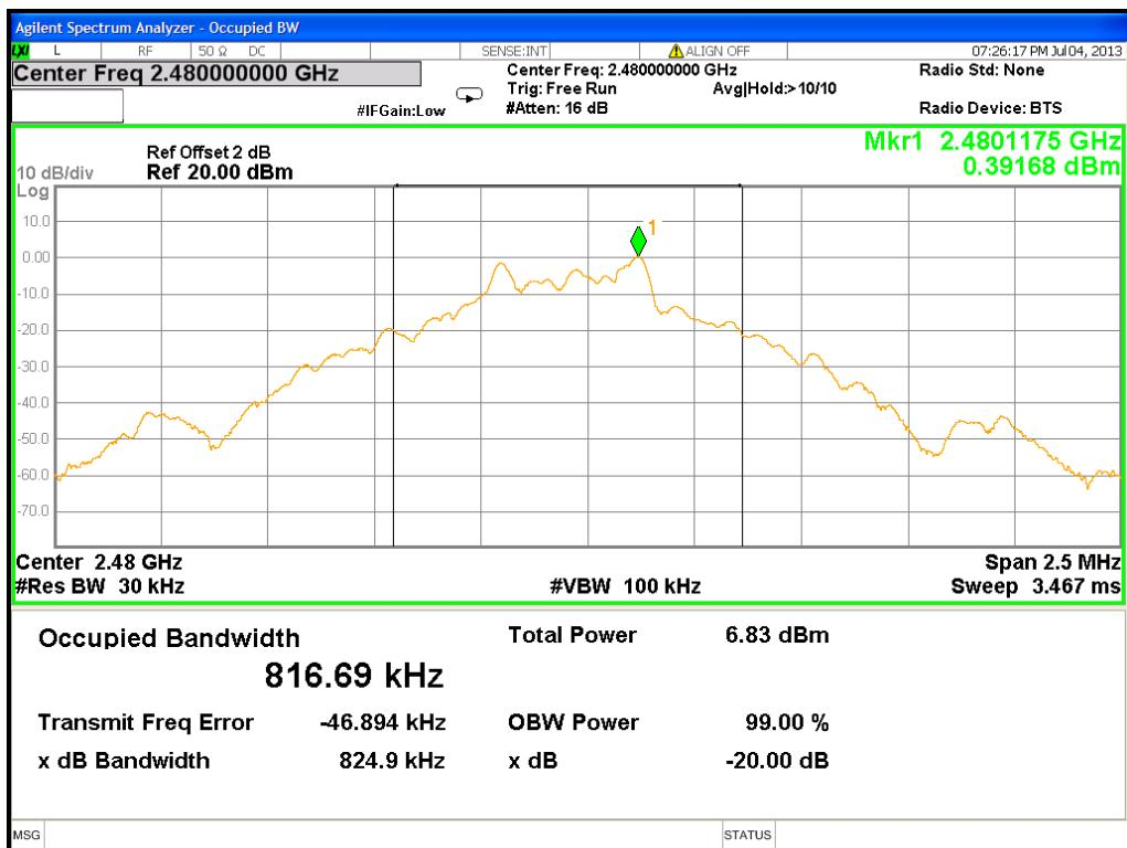
20 dB Bandwidth @  $\pi/4$ DPSK mode channel 0
