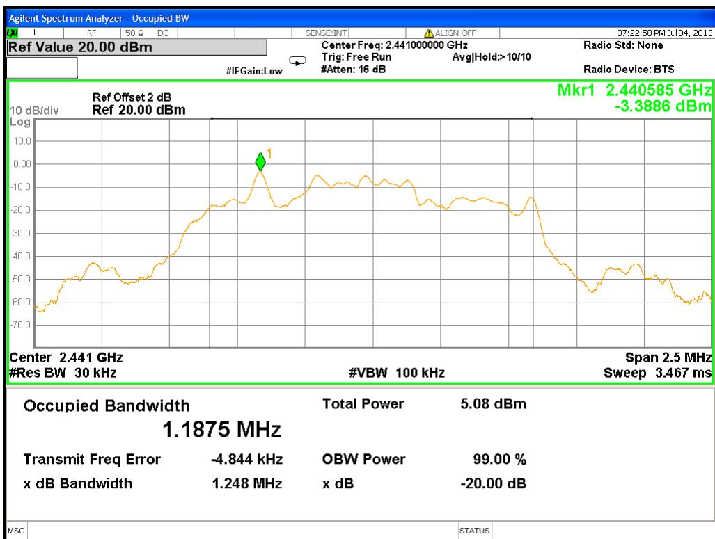
20 dB Bandwidth @ 8DPSK mode channel 78
