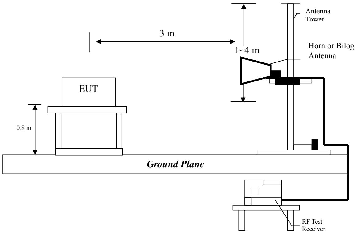
According to §15.33(a), the spectrum shall be investigated from the lowest radio frequency signal generated in the device, to the tenth harmonic of the highest fundamental frequency or to 40 GHz, whichever is lower. Spectrum Analyzer Resolution Bandwidth is 100kHz or greater for frequencies 30MHz to 1GHz, 1MHz – for frequencies above 1GHz.
