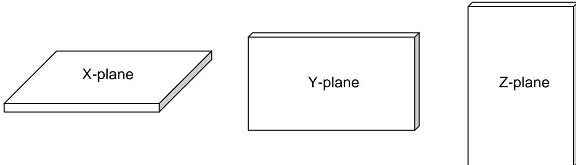
After verifying three axes, we found the maximum electromagnetic field was occurred at X-plane configuration. The final test data was executed under this configuration.
