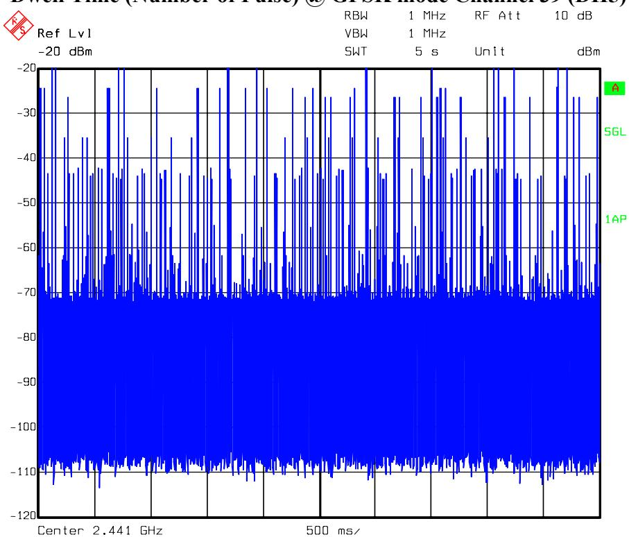
**Dwell Time (Pulse Time) @ 8-DPSK mode Channel 39 (DH1)**
