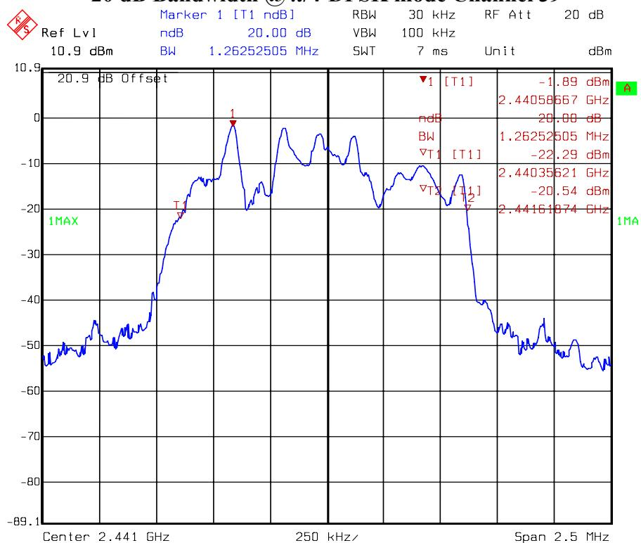
20 dB Bandwidth @  $\pi/4$ -DPSK mode Channel 78
