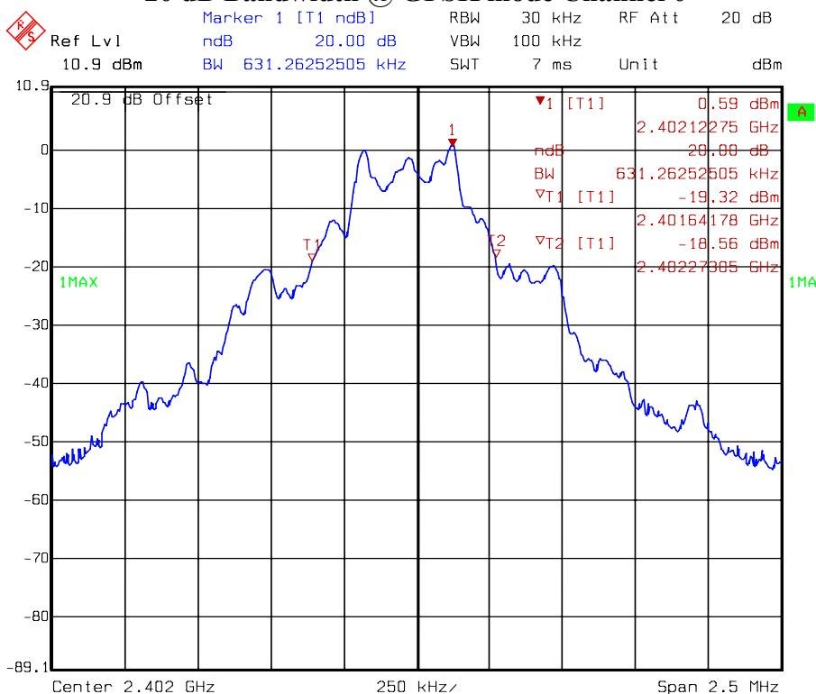
**20 dB Bandwidth @ GFSK mode Channel 39**
