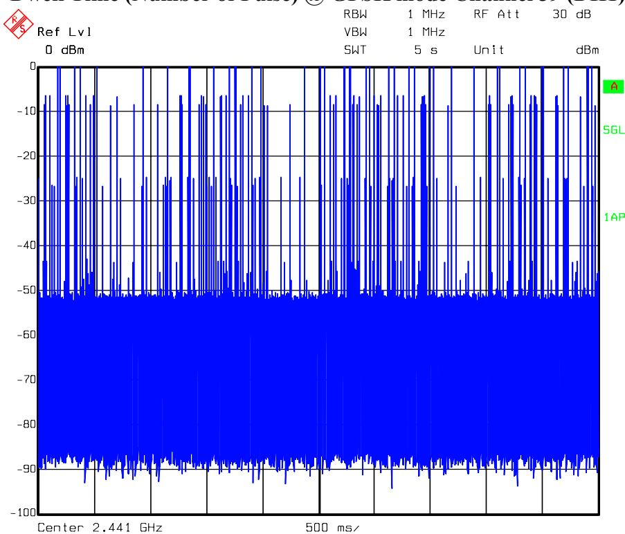
**Dwell Time (Pulse Time) @ GFSK mode Channel 39 (DH3)**
