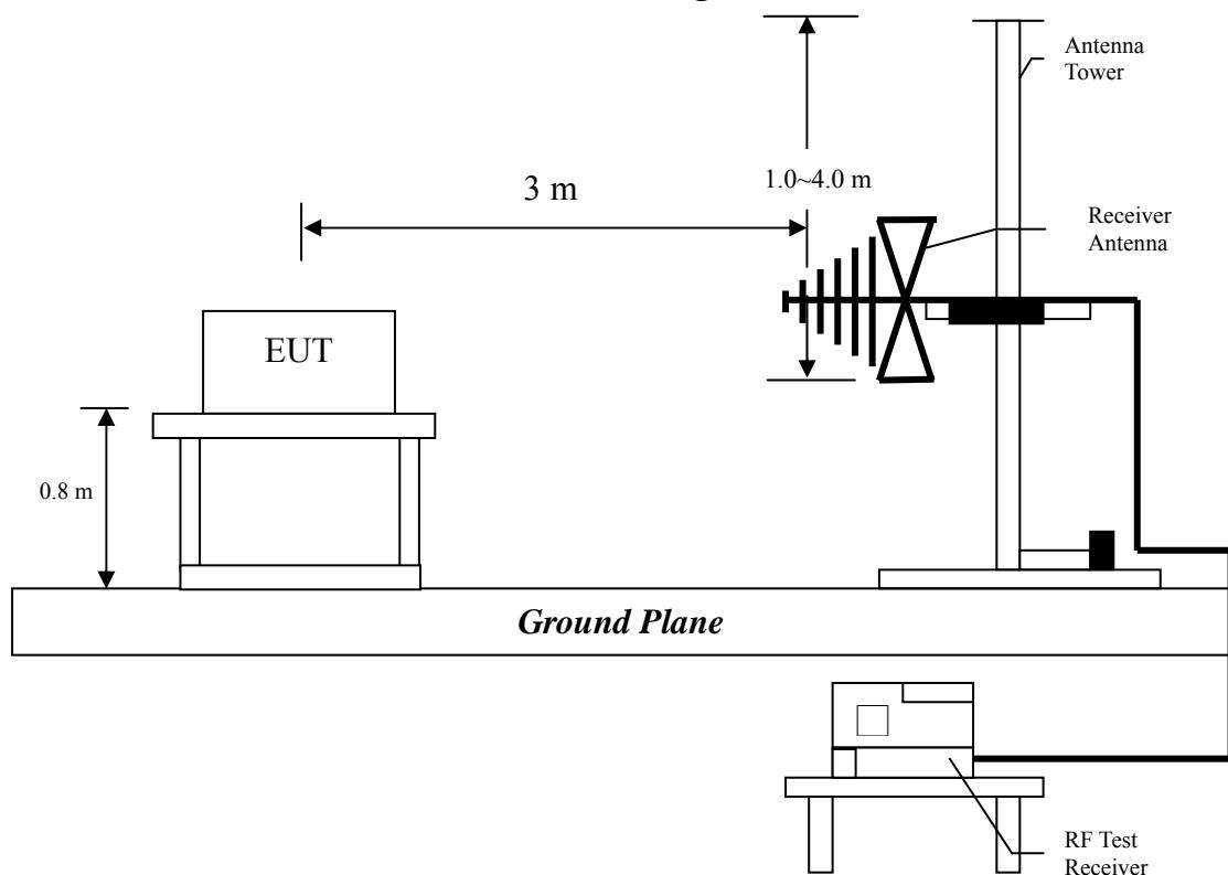
**Radiated emission above 1GHz uses Horn Antenna:**
