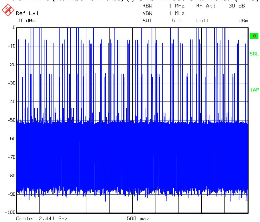
**Dwell Time (Pulse Time) @ GFSK mode Channel 39 (DH5)**
