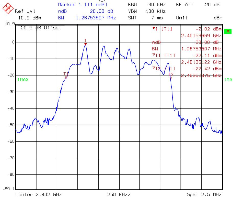
20 dB Bandwidth @  $\pi/4$ -DPSK mode Channel 39
