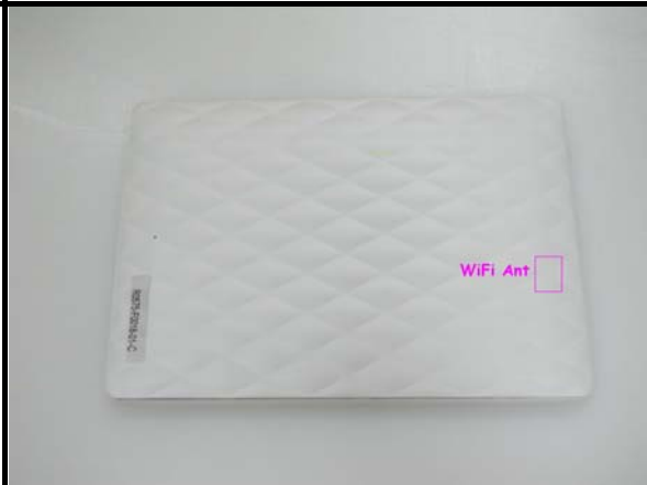
DESCRIPTION OF ANTENNA LOCATION
