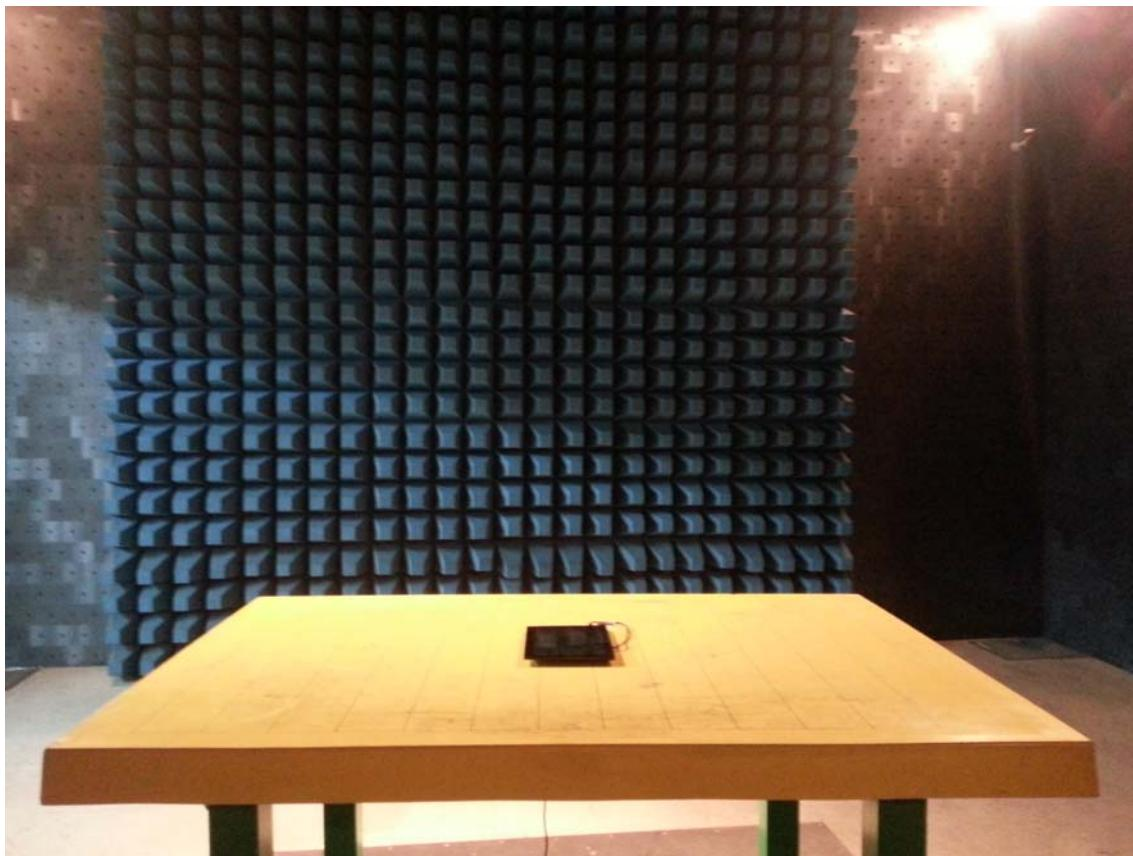
**Above 1GHz (For 2.4GHz, BT2.0, BT 4.0 Tests)**
