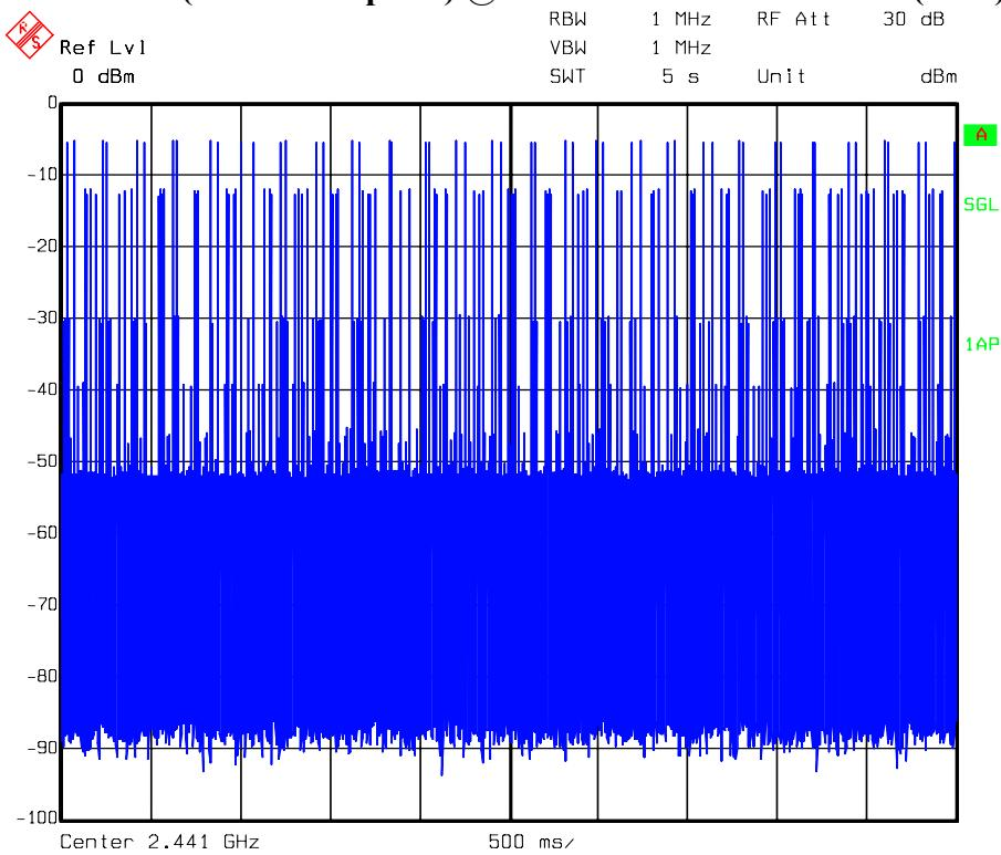
**Dwell time (Pulse time) @ 8-DPSK mode Channel 39 (DH3)**
