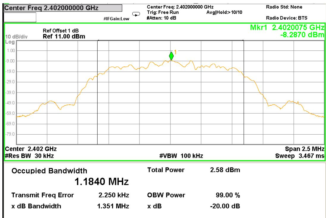
20 dB Bandwidth @  $\pi/4$ -DPSK mode Channel 39
