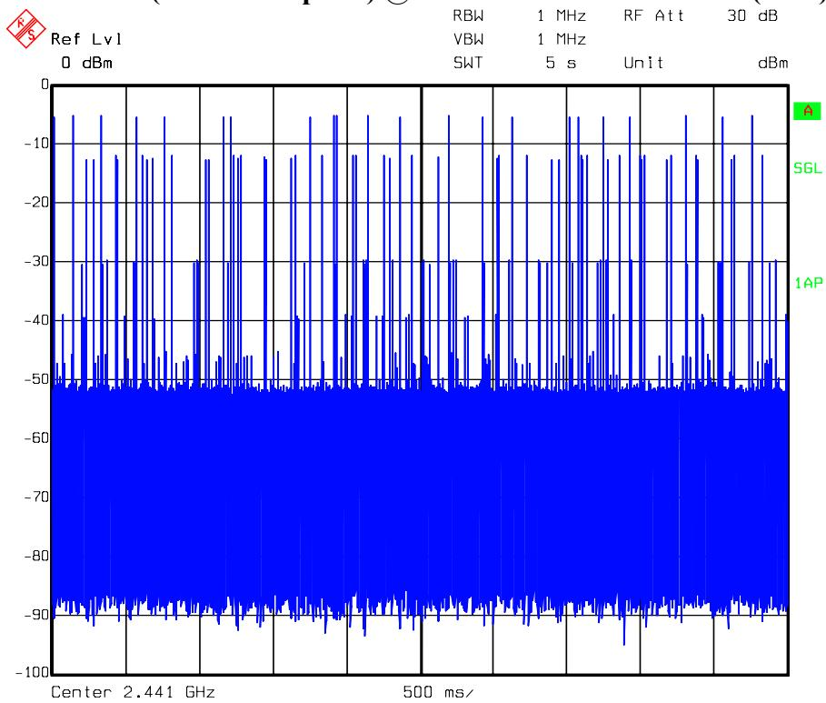
**Dwell time (Pulse time) @ 8-DPSK mode Channel 39 (DH5)**
