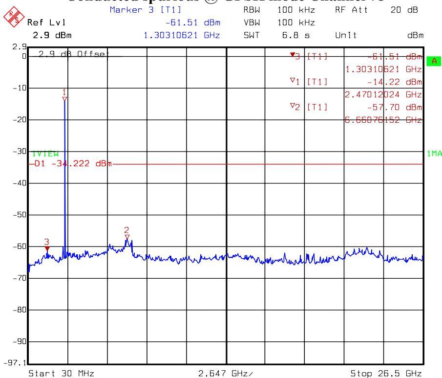
Conducted spurious @  $\pi/4$ -DPSK mode Channel 0
