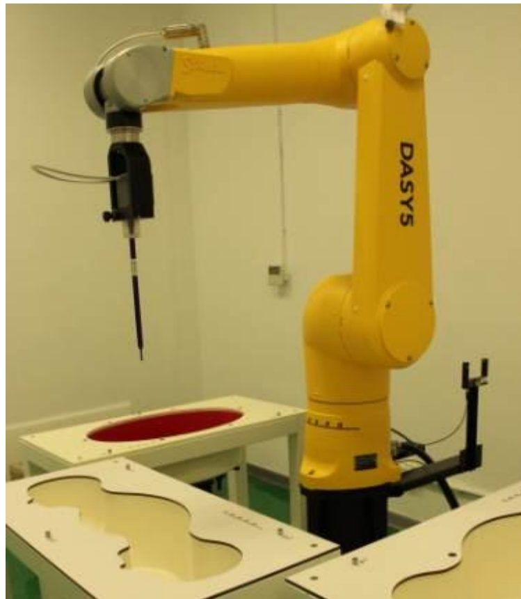
Picture 11: Specific Absorption Rate Test Layout
