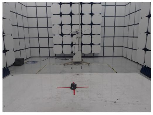
RADIATED EMISSION TEST SETUP ABOVE 1GHz
