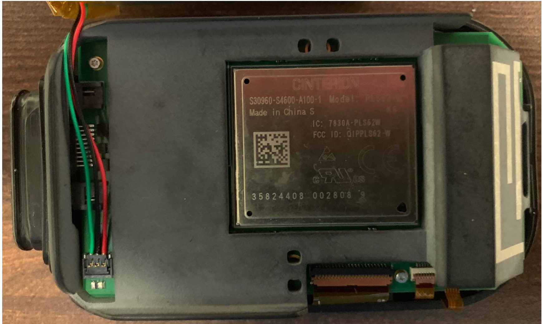
Exhibit: Internal Photos (Interior with Battery Removed) (FCC ID: ZIMH40L; EUT IC ID: 9647A-H40L)
