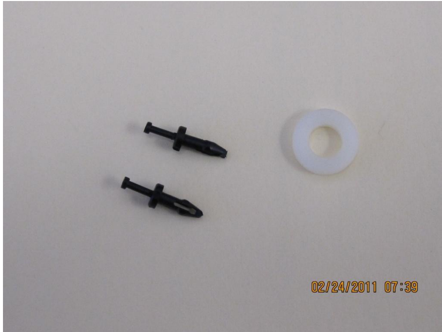
FASTEX Pins to mount PCB, Washer for Antenna
