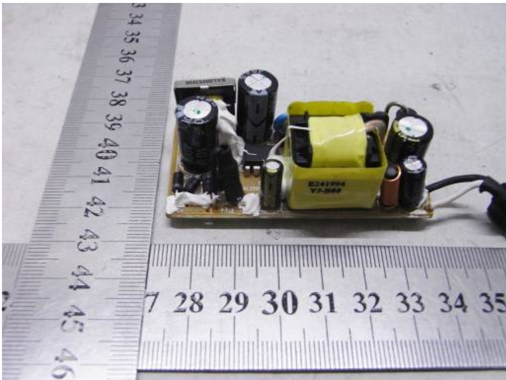
INTERNAL PHOTO OF POWER SUPPLY-1
