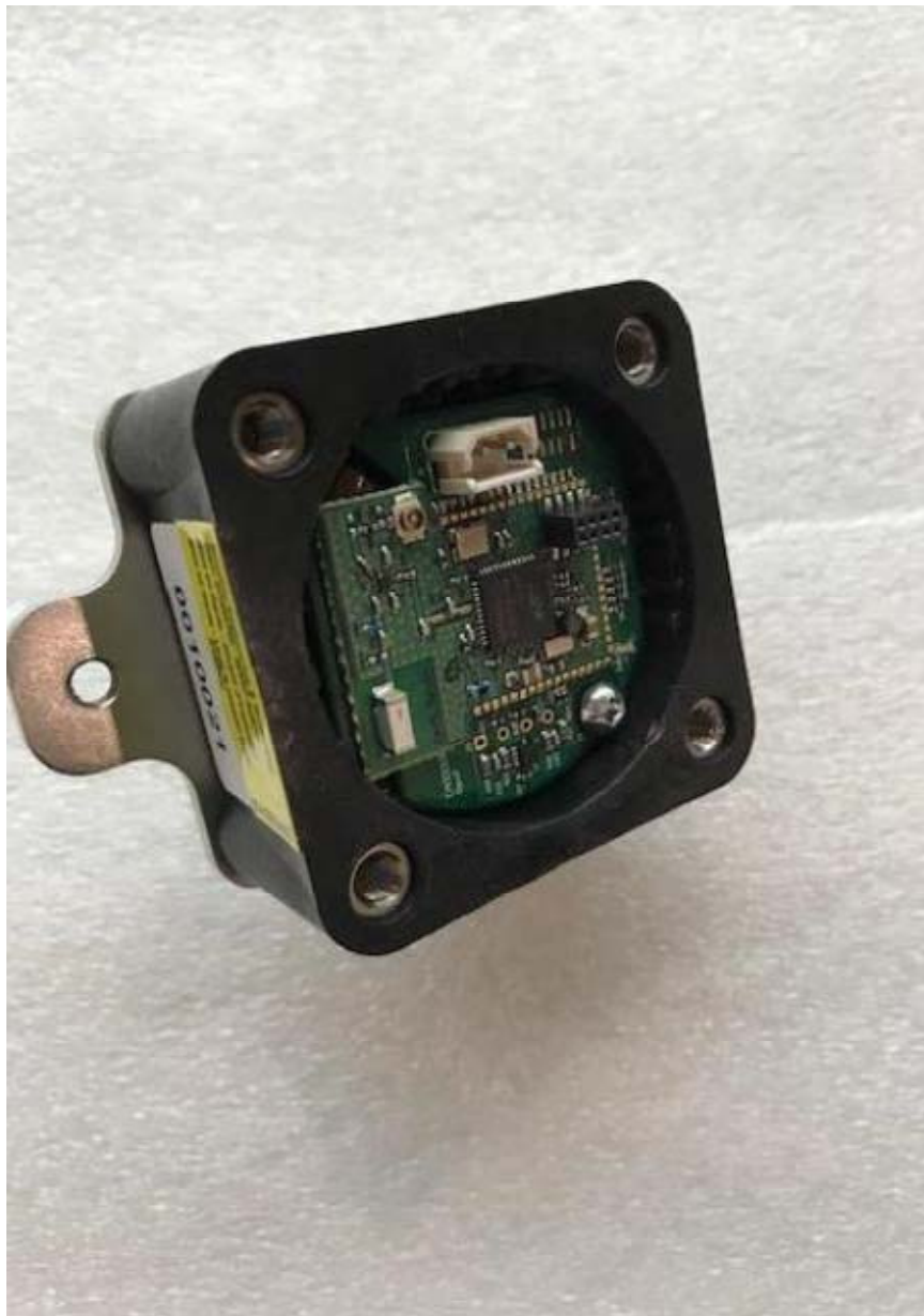
Figure E22A.1 – Internal Photo – Host 1 Battery Removed
