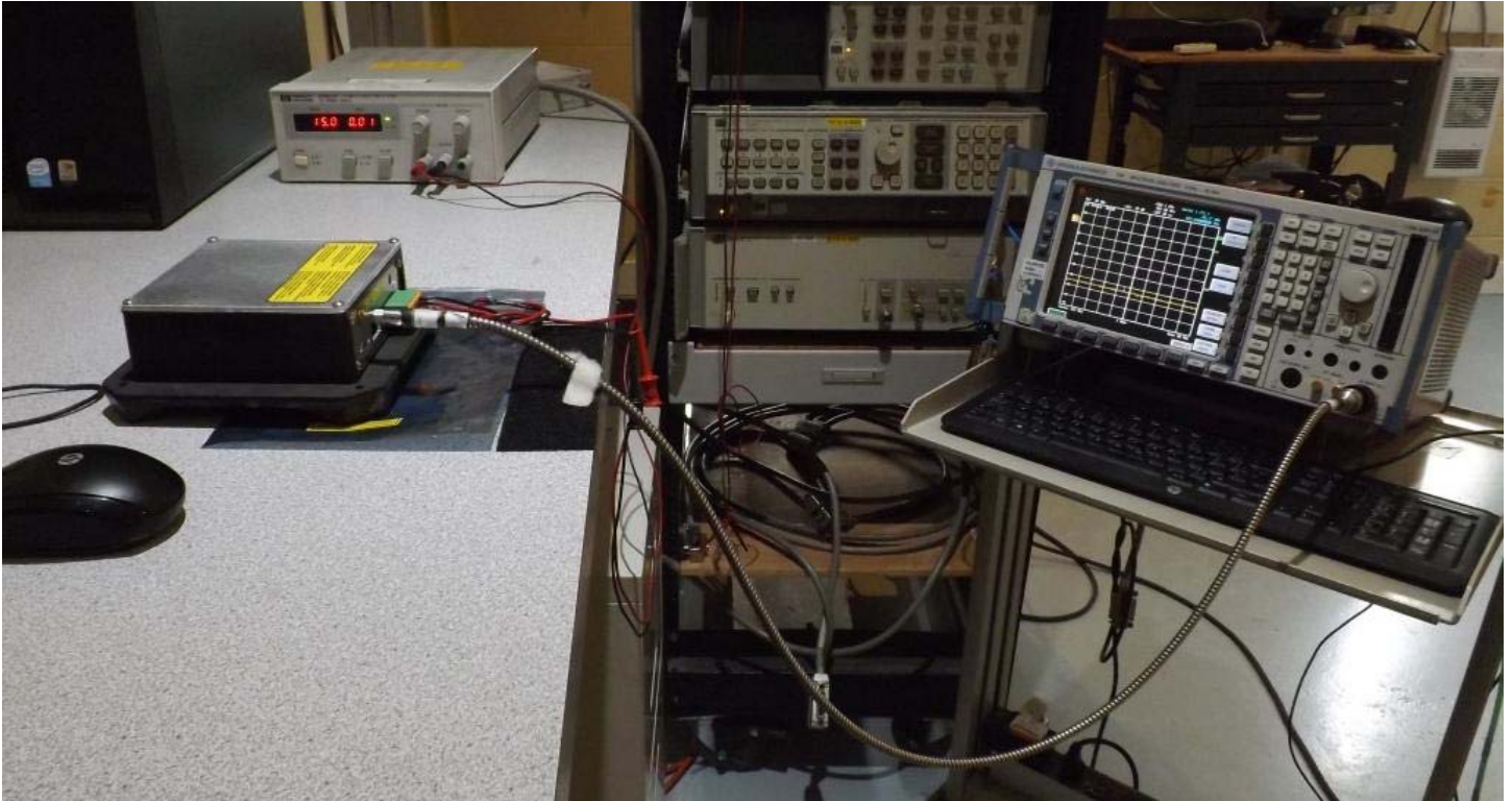
Figure E12.1 – Setup, Antenna Port Conducted
