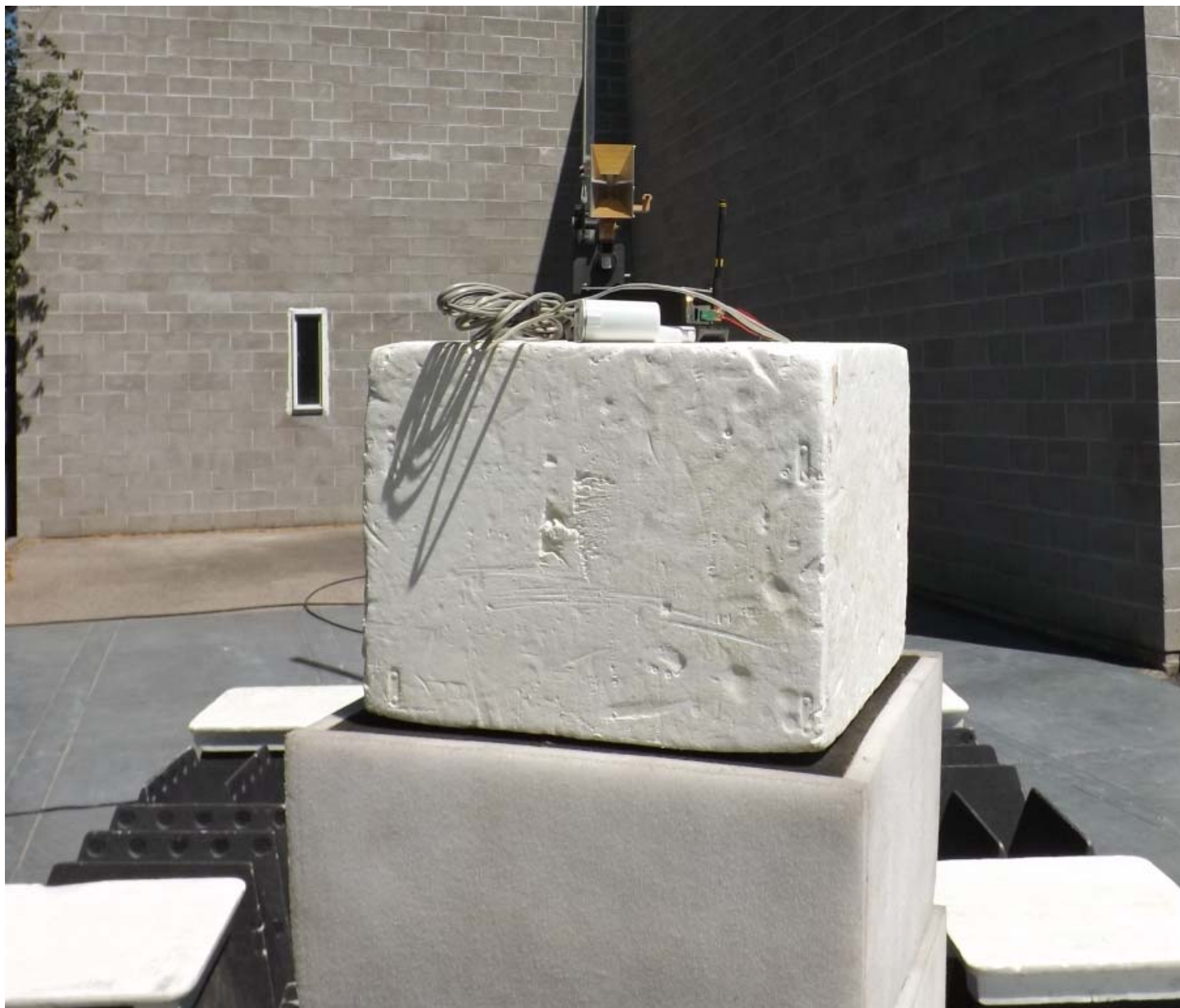
Figure E12.3 – Setup, Radiated Tx, 1 – 10GHz
