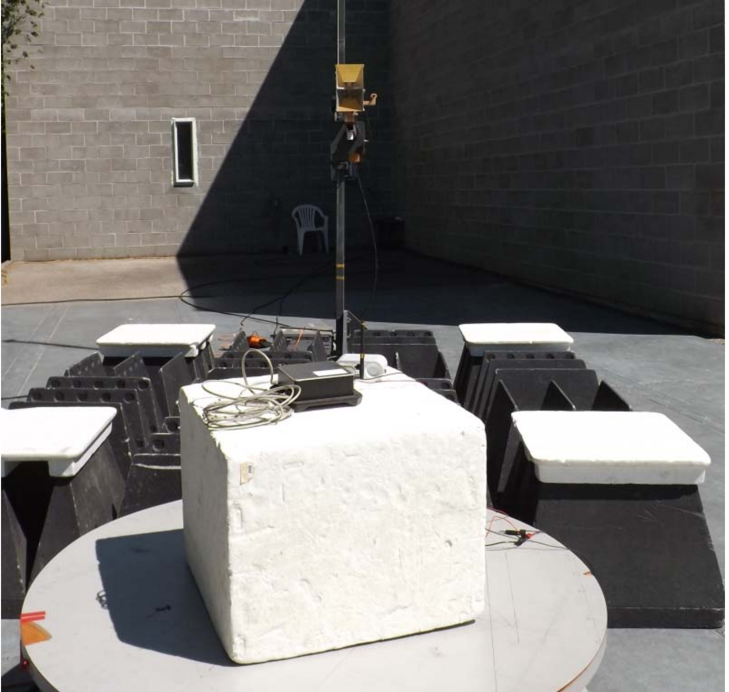
Figure E12.4 – Setup, Radiated Rx, 1 – 5GHz
