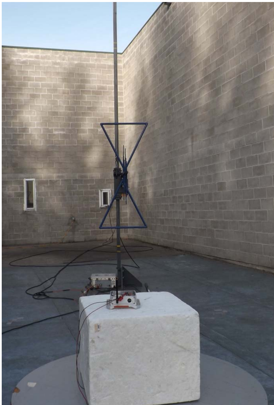
Figure E25.6 – Radiated Measurements 30 – 1000MHz, Vertical
