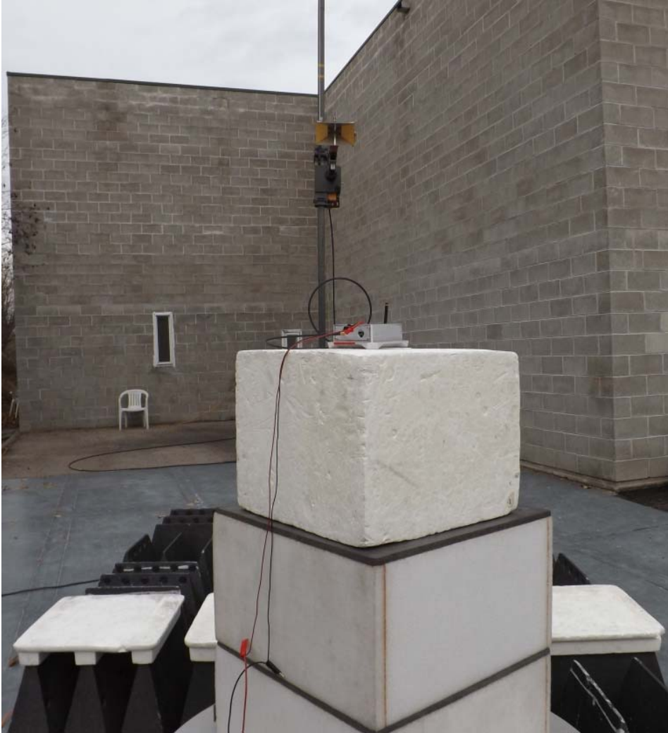
Figure E25.8 – Radiated Measurements 1 – 18GHz, Vertical
