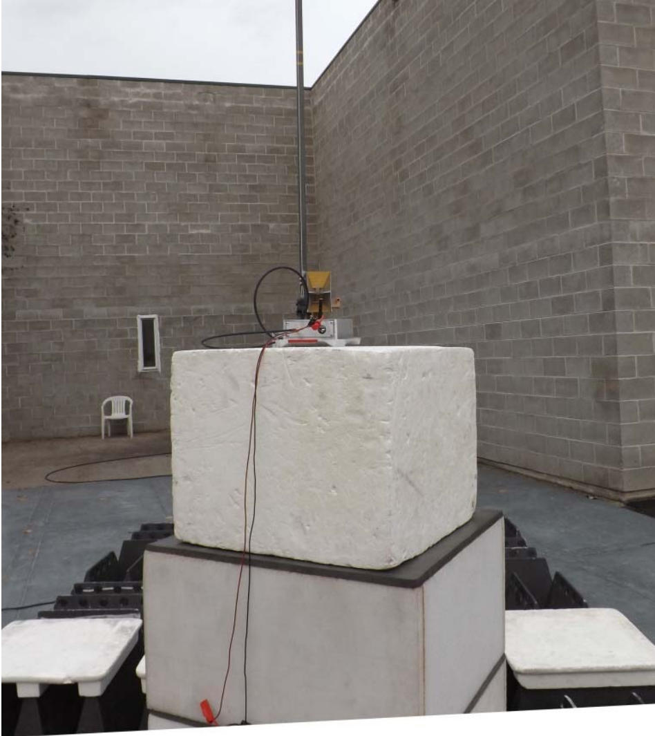
Figure E25.7 – Radiated Measurements 1 – 18GHz, Horizontal
