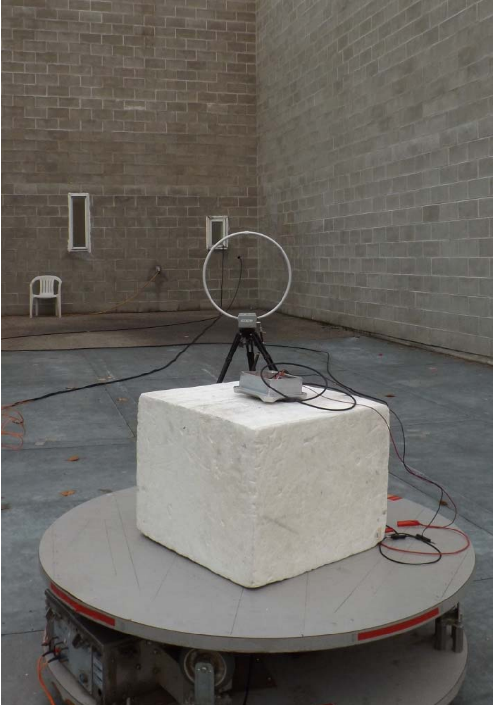
Figure E25.3 – Radiated Measurements 9kHz – 30MHz, Front Polarization
