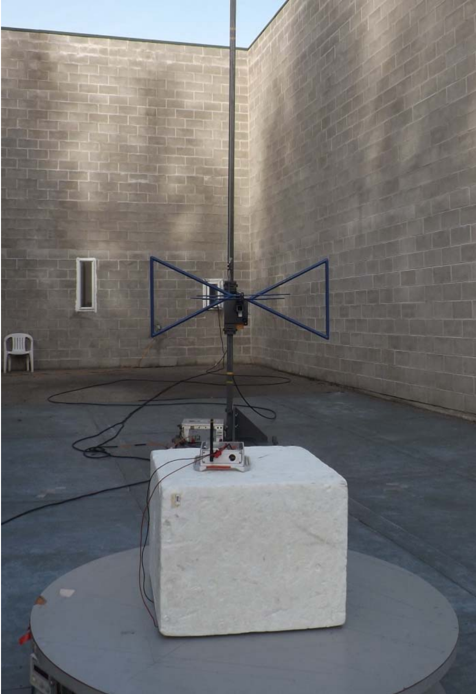
Figure E25.5 – Radiated Measurements 30 – 1000MHz, Horizontal
