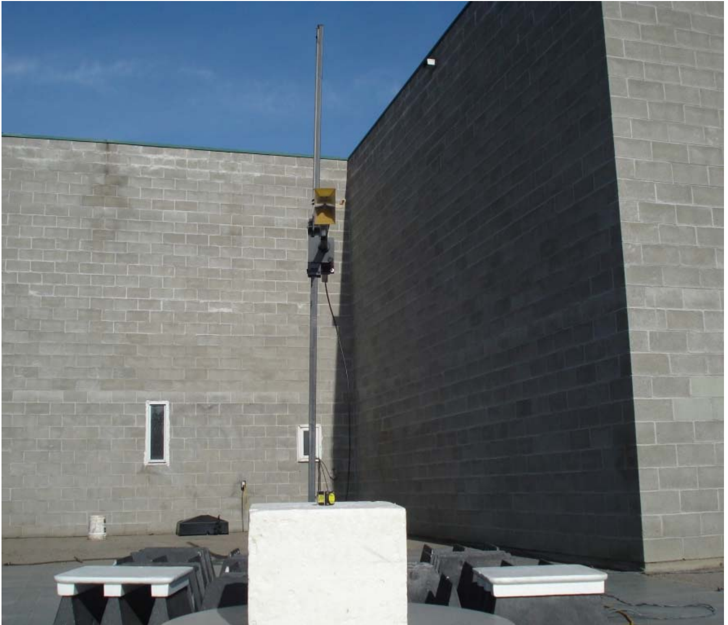
Figure 3 – Emissions Test w/ Double Ridge Horn 1-18GHz
