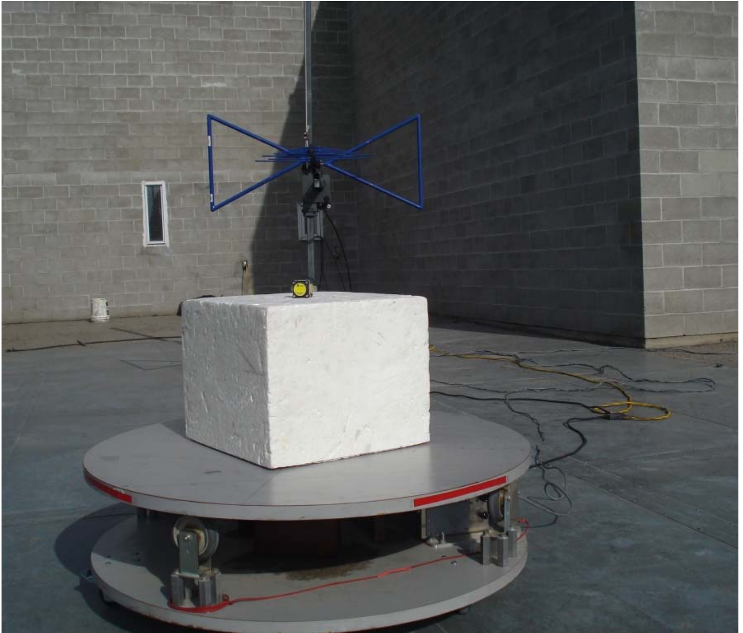
Figure 2 – Emissions Test w/ Chase Bilog Antenna 30-1000MHz
