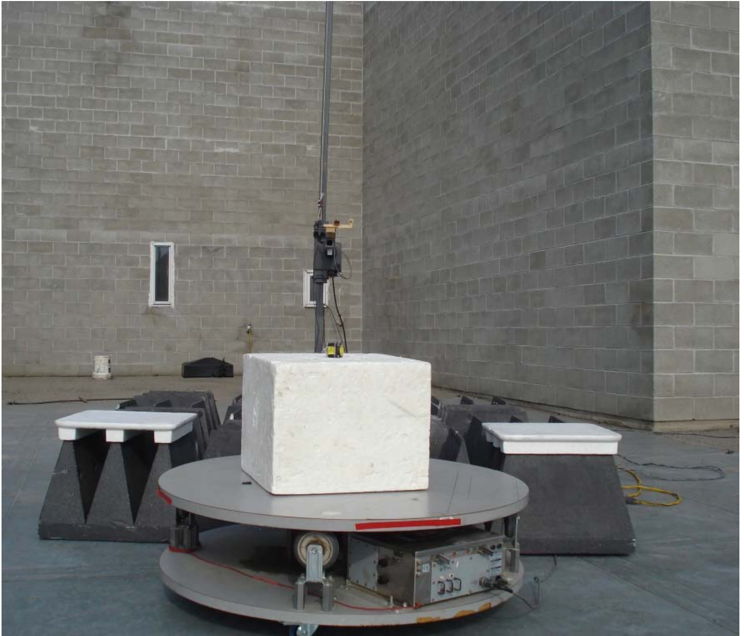
Figure 4 – Emissions Test w/ Standard Gain Horn 18-26.5GHz
